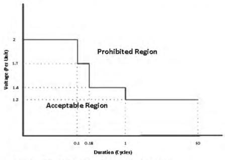
Figure 1: IEEE Transient Over Voltage Tolerance Curve
