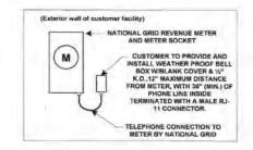
Figure 1B – Outdoor Meter Installation not to scale
