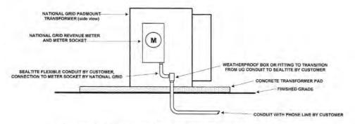
Figure A- 1: Revenue Meter Phone Line Installation Guide
